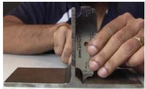
Fillet Welding Check
